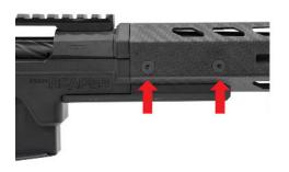
(4) HAND GUARD SCREWS | 1/8" ALLEN HEAD (2) ON EACH SIDE OF HANDGUARD
